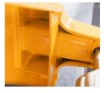
Extra reinforcement rod on top of the chassis.
